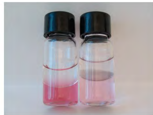
Fig. 1 Digital photograph of a 40 nm gold colloid covered with hexane without (left) and with the addition of 28.6 vol.% of ethanol (right).
